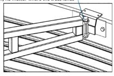
Strong, robust, galvanized square hollow section tube construction used for bottom chord as well as top chord of truss and also for verticals
