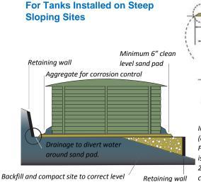
Inert rock aggregate must be placed around the base (circumference) of your tank after installation.
